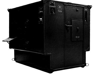
The AN/TRC-115 contains the necessary units to control, switch and operate remote telephone line, remote teletype-writer, and the local operator's equipment. The unit consists of a communication control console, one radio receiver, one radio transmitter, two radio set controls, one antenna coupler and coupler control, and a telegraph terminal group.
