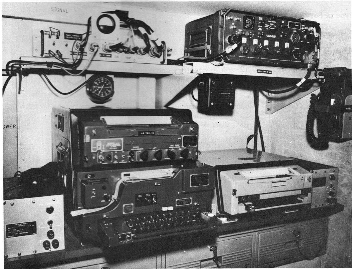
Figure 96. Radio Teletypewriter Set AN/GRC-142, curb-side view.
