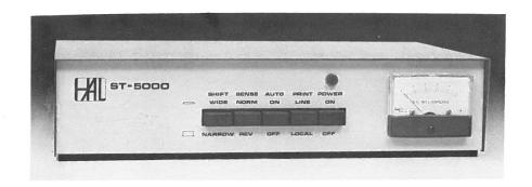
The HAL ST-5000 Demodulator provides excellent, reliable RTTY performance on both HF and VHF bands. Features such as a hard limiting front end, active discriminator, and active detector make this unit a big value. Wide and narrow shift (850 hz and 170 hz), normal or reverse sense, autostart, self-contained high voltage loop supply, and an audio tone keyer are standard.
