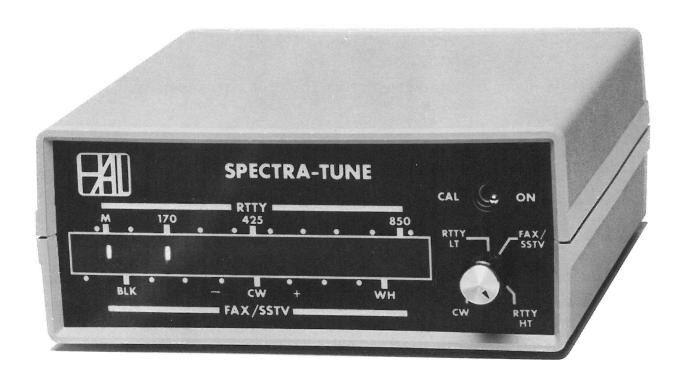
The HAL SPT-1 SPECTRA-TUNE® Multi-Mode Tuning Indicator permits quick and accurate tuning of RTTY-High Tones, RTTY-Low Tones, Facsimile (FAX), Slow-Scan Television (SSTV) and Morse Code (CW) signals. The frequency spectra of the received signal is displayed on a calibrated 40-segment red LED bar graph. The front panel calibration control allows the selection of which 1000 HZ range from 300 HZ to 3000 HZ is to be displayed. The unit instan-
