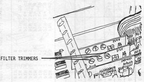
( ) Adjust the Audio Signal Generator for 2295 Hz (HI-TONES SPACE).
