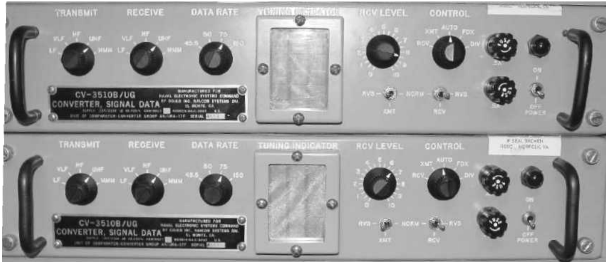
AN/URA-17F converter/keyer– Comprised of two CV-3510B/UG converters in an enclosure.
