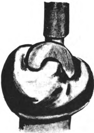
COLD SOLDER JOINT
