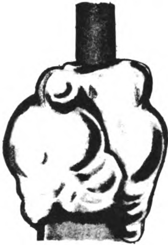
EXCESSIVE SOLDER JOINT
