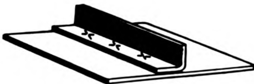
PANEL WITH SPOT-WELDED STIFFENING RIB
