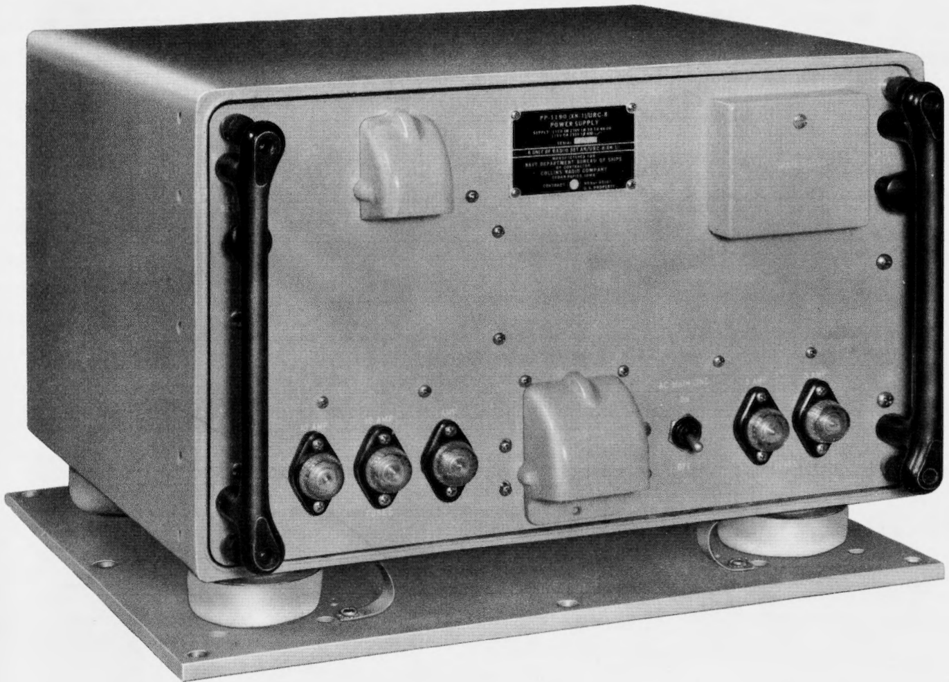
Figure 1-7. Power Supply PP-1190(XN-1)/URC-8
