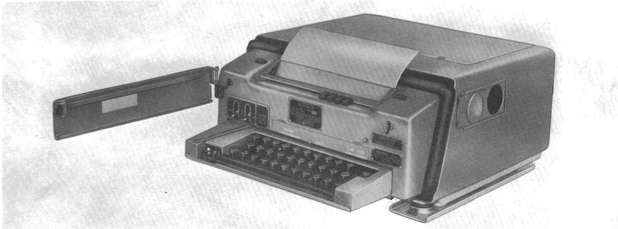
C. Installed in Shock-Mounted Non-Tactical Case CY-2977A/UG
