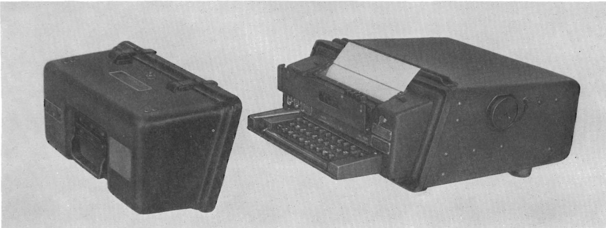
B. Typical Installation in Tactical Case CY-2976/PG (Case not shock-mounted; copy holder closed.)
