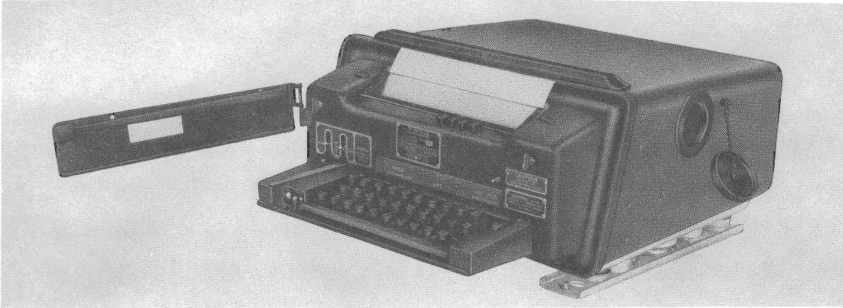
A. Installed in Shock-Mounted Tactical Case CY-2976/PG
