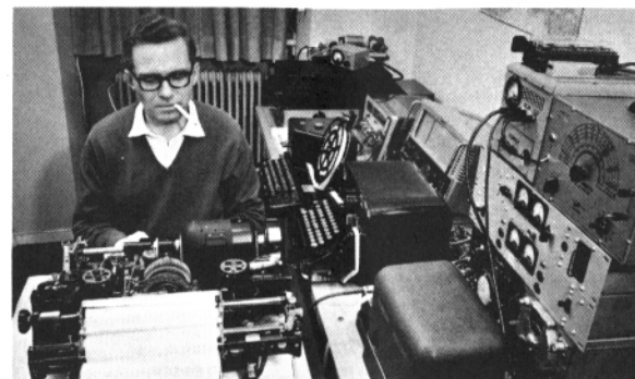
Transmitter, HX-20; P.A., 4-EL 34 In grounded grid; Receiver, Eddystone 888a; Terminal Unit, FSR 1. (AP66862); Input Filter, W4EHU Comb. Filter; Tuning Indicator, Cross Line. Teletype Equipment: Creed 7B Page Printer; Siemens T 68 Tape Printer; Teletype Model 14 TD; Siemens T Loch 1M Key-board Perforator.
