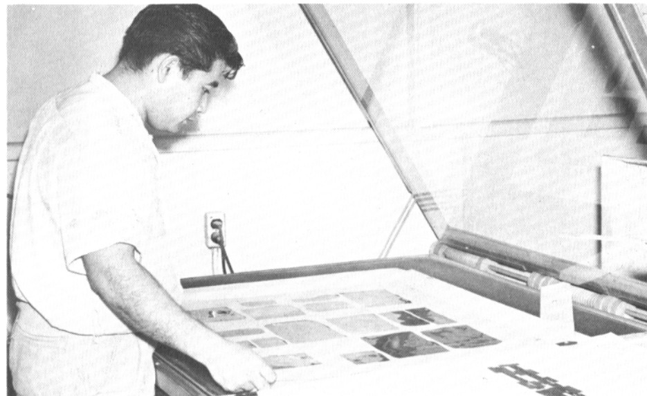
The resulting negatives are placed in another easel with special sensitized material which form the final printing plates for the printing press.
