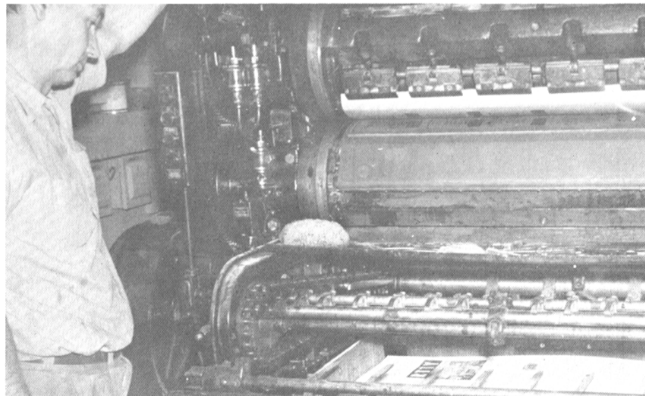
RTTY Magazine goes to press! This is called "offset printing," a method extensively used for small-volume printing of periodicals, circulars, bulletins, and the like.
