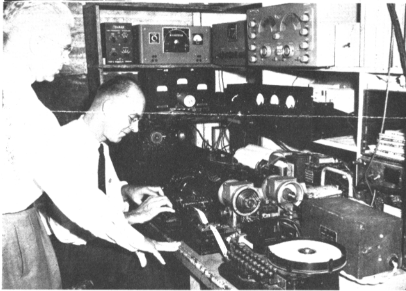
SCRAP EQUIPMENT, purchased in search through war surplus stores, was cleaned up, overhauled, and adapted for receiving Teletype signals by radio. Ray Morrison, seated, demonstrates equipment to Steve Janiszewski (1210).
