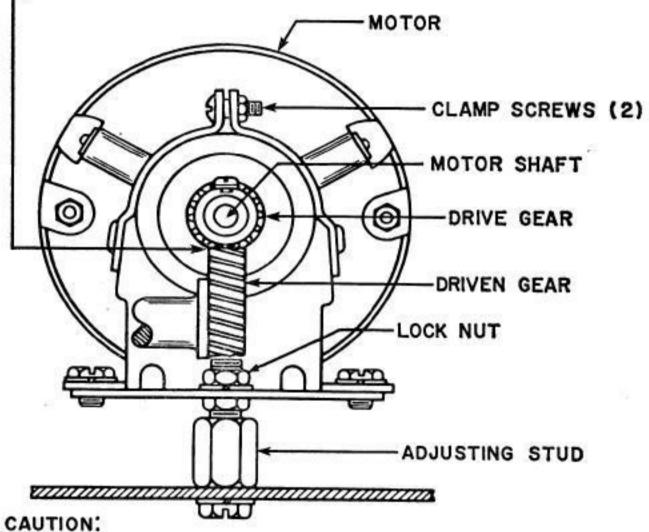
IF MOTOR BECOMES BLOCKED FOR SEVERAL SECONDS, THERMAL CUT-OUT SWITCH WILL BREAK CIRCUIT. SHOULD THIS HAPPEN, ALLOW MOTOR TO COOL AT LEAST 5 MINUTES BEFORE DEPRESSING RED RESET BUTTON.
