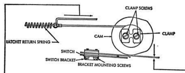
(B) RATCHET DRUM ASSEMBLY RETURN SPRING REQUIREMENT
