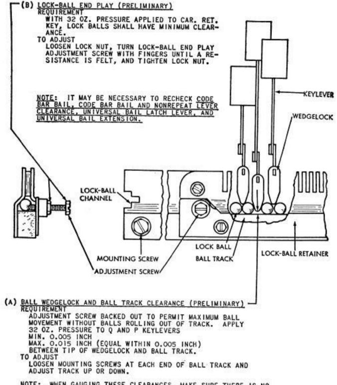
NOTE: WHEN GAUGING THESE CLEARANCES, MAKE SURE THERE IS NO CLEARANCE BETWEEN LOWER EDGE OF CODE LEVER EXTENSION AND BOTTOM OF SLOTS IN WEDGES.
