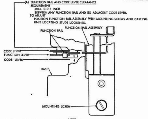
NOTE THIS ADJUSTMENT SHALL NOT BE MADE UNLESS THE LOCK-BALL CHANNEL HAS BEEN DISASSEMBLED.
