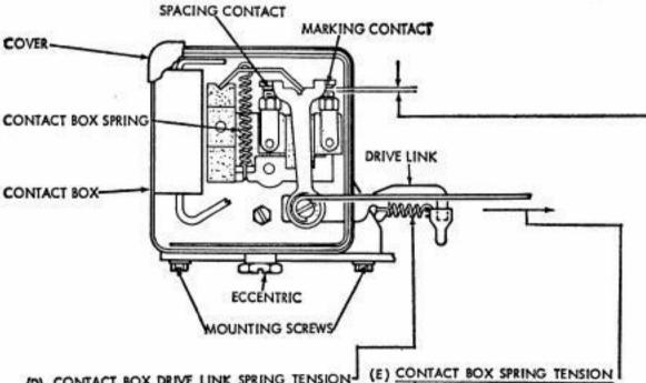
(D) CONTACT BOX DRIVE LINK SPRING TENSION
