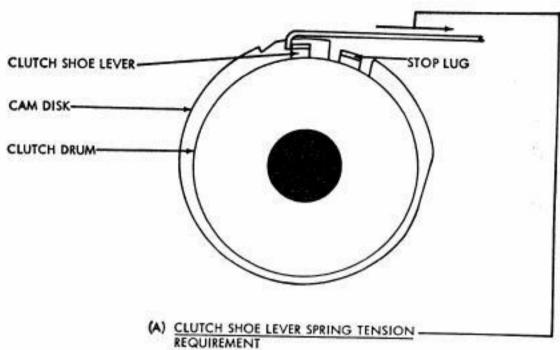
CLUTCH ENGAGED. CAM DISK HELD TO PREVENT TURNING MIN. 15 OZS. MAX. 20 OZS. TO MOVE SHOE LEVER IN CONTACT WITH STOP LUG.
