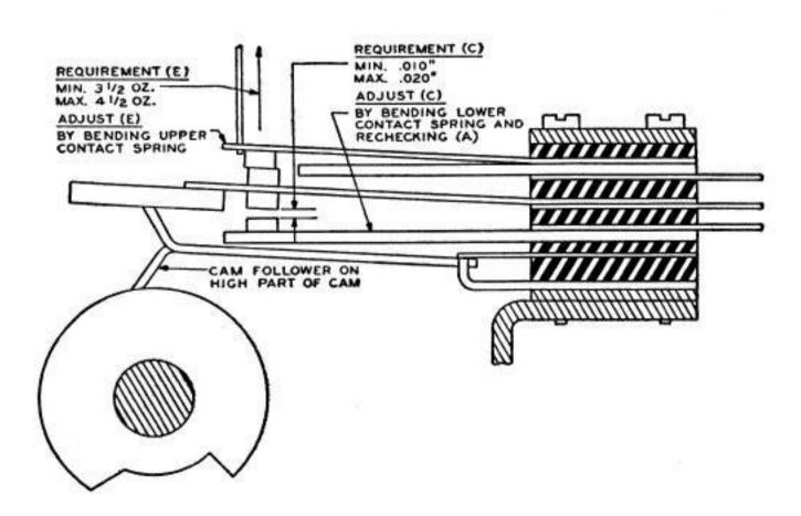
New-Style TP116962 Contact Assembly (with lower TP-84705 contact spring and TP105940 stiffener)
