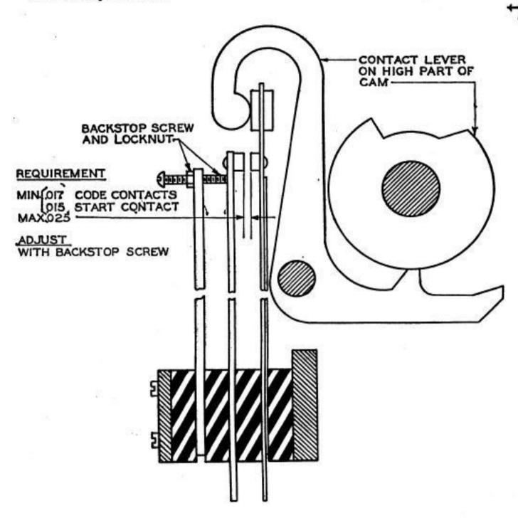
Note: The requirement given in this figure applies when a distortion test set is available for checking signals. If no distortion test set is available, contact gap requirements should be as follows:
