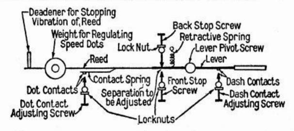
The proper maintenance of these keys in accordance with the following instructions is necessary to insure good telegraph service.
