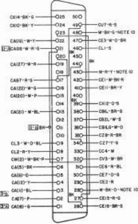
CN CONNECTOR RECEPTACLE - 50 PT. 182733
