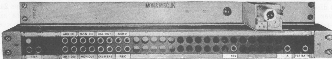
Fig. 10 – 2400- or 2600-cycle Signal Monitoring Unit
