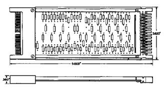
Consists of component apparatus mounted on a printed wiring board equipped with a P-42F226 terminal block on one end and a P37C859 connector on the other end. Initially used in No. 1 ESS.
