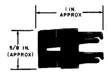
A 2-terminal quick clip connector with a spring clasp on one side which fits over two adjacent clips of a 66-type block. A molded plastic block is fitted around the middle to provide a working surface for the 714-type tool.
