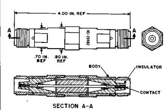
A male, coaxial adapter arranged for screw-on connection at both ends to a KS-14317 L3 plug. For use in testing and fault-location work in L1, L3, and L4 Carrier Systems.
