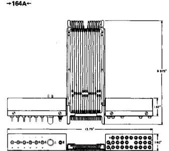
Consists of jacks, switches, and a lamp mounted on a metal mounting plate with terminal covers. A printed wiring board that contains eyelets used for plugging into the circuit is also assembled to the metal frame. Intended for use as an extender board and as an aid in locating faulty circuit pack of No. 101 ESS. Initially used in the 124A test set.
