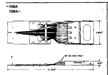
Each consists of a printed wiring board and a 905B connector assembled in a metal frame. The 158A has permanent connections between wiring board and 905B connector. The 159A has connections between wiring board and 905B connector which can be interchanged to permit a variety of tests. Intended for use in No. 1 ESS to permit printed wiring boards mounted in 36A apparatus mounting to be extended beyond the apparatus mounting for testing purposes.
