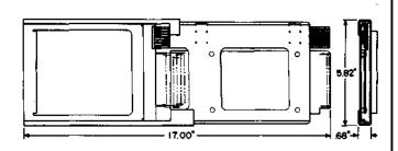
Consists of a steel framework equipped with sliding adjustable keys which mount into a 927-type connector. Intended for use in extending AR-coded circuit packs from their normal mounting positions in the 58A, 59A, and 61A apparatus mountings for in-circuit testing. Initially used in No. 1 ESS (ADF).
