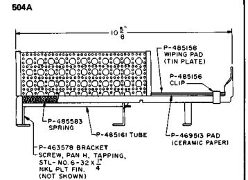
Soldering copper holder. Designed to clamp on rolling ladder steps. May also be used with ED-92008-01 mounting bracket or on a flat surface. See the 721A tool for adapter which may be added to this tool for holding KS-14440 and KS-16346 soldering coppers. This adapter cannot be used with KS-8740 soldering copper. Also see Rest, Copper, Soldering, Section 074-253-130. For general use.
