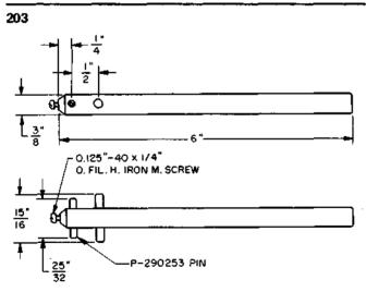
Index wheel holder. For use on A- and B-type sequence switches and 155A and 157-type interrupters.
