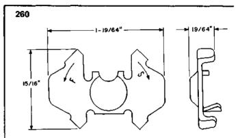
Dial governor holder. For use in holding rotating parts of 2-, 4-, and 5-type dial governors stationary when adjusting them for speed.
