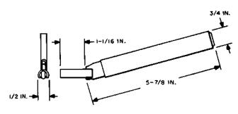
Relay core holder. For use on U-, UA-, and Y-type relays having hinge pin-type armature suspension.
