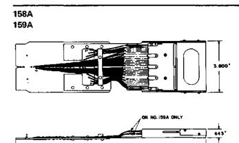
Each consists of a printed wiring board and a 905B connector assembled in a metal frame. The 158A has permanent connections between wiring board and the 905B connector. The 159A has connections between wiring board and the 905B connector which can be interchanged to permit a variety of tests. Intended for use in No. 1 ESS to permit printed wiring boards mounted in the 36A apparatus mounting to be extended beyond the apparatus mounting for testing purposes.
