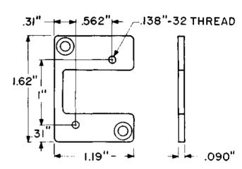
A metal U-shaped plate arranged to mount a 263A jack mounting in positions intended for mounting a 212A jack mounting. Intended for use in common systems.
