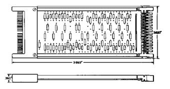
Consists of component apparatus mounted on a printed wiring board equipped with a P-42F226 terminal block on one end and a P37C859 connector on the other end. Initially used in No. 1 ESS.
