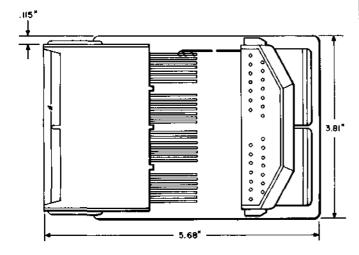
Consists of a printed wiring board and a 905B connector assembled in a metal frame. Intended initially for use in the No. 1 ESS to permit testing of the trunk unit relays of the plug-in type trunk units.
