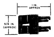
A two-terminal quick clip connector with a spring clasp on one side which fits over two adjacent clips of a 66-type block. A molded plastic block is fitted around the middle to provide a working surface for the 714-type tool.
