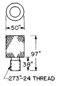
A metal adapter arranged to thread into a 413-type plug. Intended for use in testing cable pairs on main distributing frames equipped with 300-type connectors.
