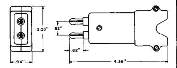
A twin plug and twin jack arranged for use with a 240 or similar-type jack and a 419A plug. Each finger provides sleeve contact only. Intended for use as a monitor plug adapter in E6 telephone repeaters of common systems.
