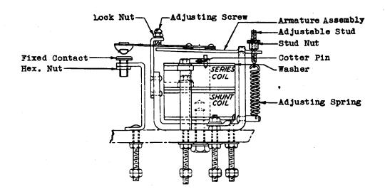
FIG. 2 - SECTIONAL VIEW - REVERSE CURRENT RELAY
