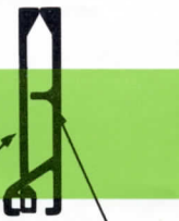
153643 Slide — Spans the 153795 slide — May be operated by one or two function levers
