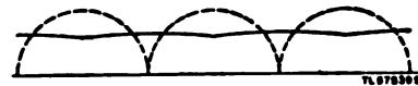
Figure 207. Output waveshapes of simplified rectifier circuit with choke coil and capacitors connected.
