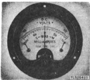
Figure 119. Meter of Switchboard BD-100 with correct position of meter needle for zero bias.
