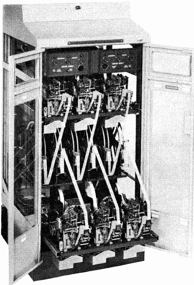
Figure 4-59. Model 28 Typing Reperforator Monitor Group (Front Doors Open)
