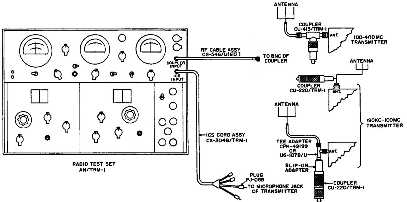
Figure 2-3. Typical Connections for Radio Transmitter Performance Tests
