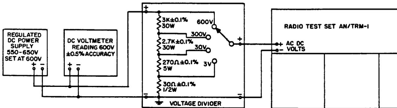
Figure 11-1. Set-up for Performance Test of DC Voltmeter
