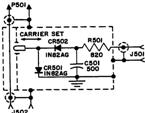
Figure 4-8. R.F. Coupler-Detector CU-413/TRM-1, Schematic Diagram
