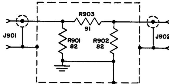
Figure 4-5. Fixed Attenuator CN-287/TRM-1 (12db), Schematic Diagram
