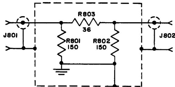
Figure 4-6. Fixed Attenuator CN-399/TRM-1 (6db), Schematic Diagram
