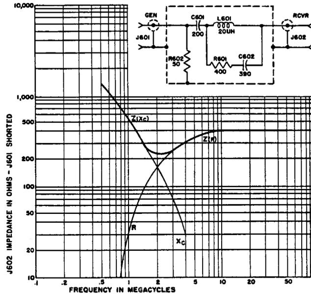
Figure 4-3. Test Adapter MX-1652/TRM-1, Schematic Diagram and Input Impedance-Frequency Curve (Antenna Simulator)
