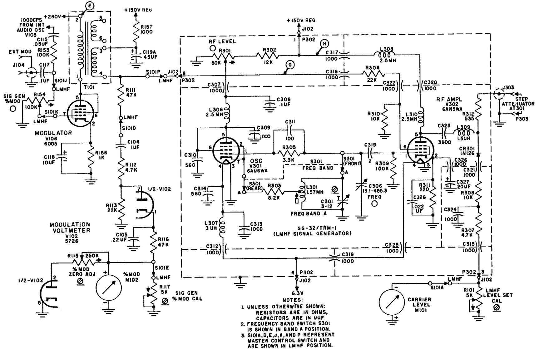
Figure 4-1. Signal Generator SG-32/TRM-1, Simplified Schematic Diagram
