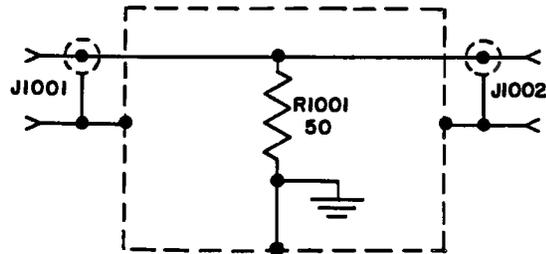
Figure 4-4. Test Adapter MX-2079/TRM-1 (50 ohm termination); Schematic Diagram
