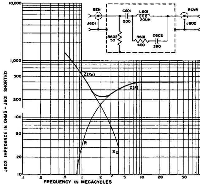
Figure 2-2. Test Adapter MX-1652/TRM-1, Input Impedance/Frequency Curve
