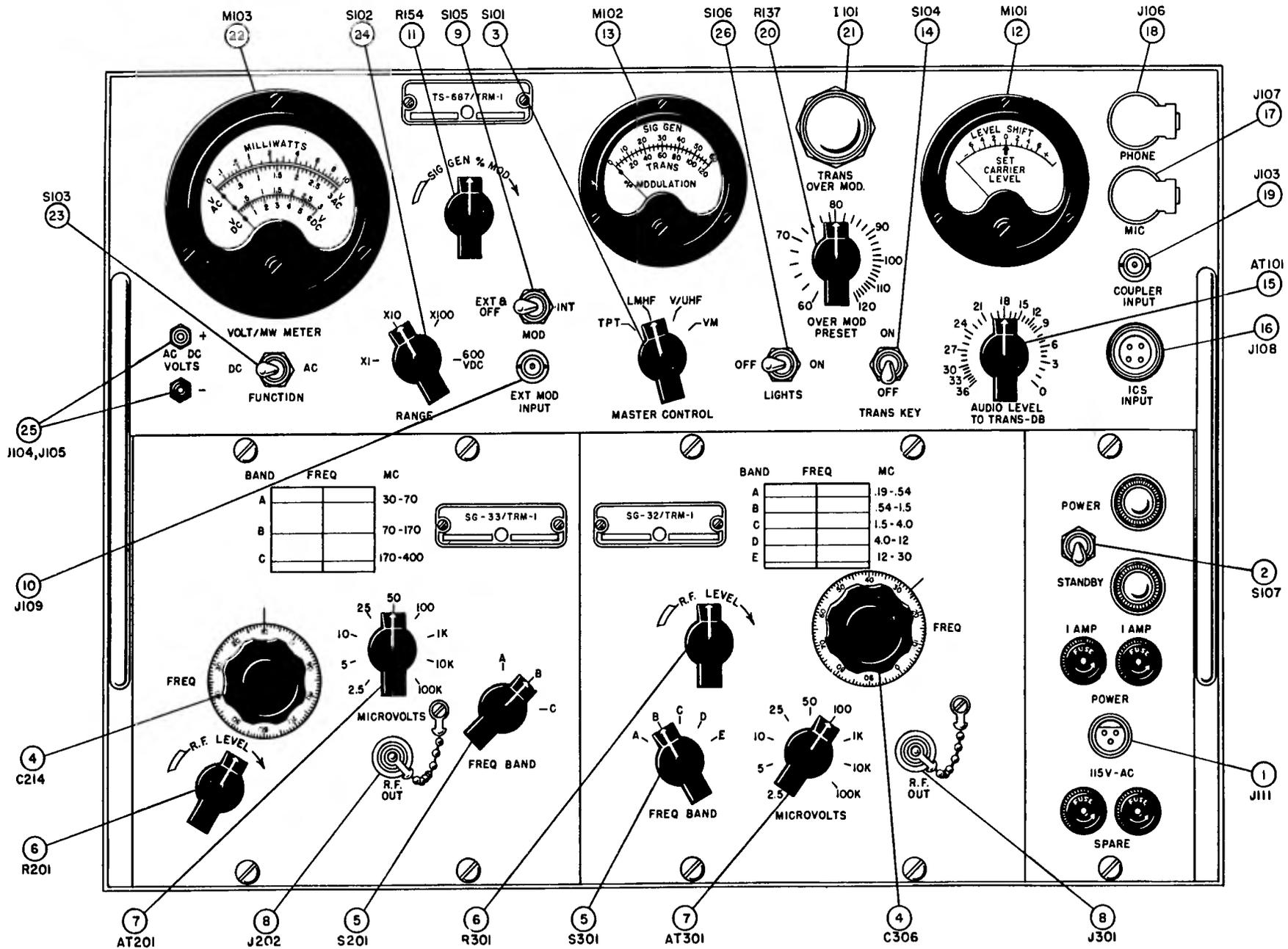
Figure 2-1. Operating Controls and Connectors, Radio Test Set AN/TRM-1
