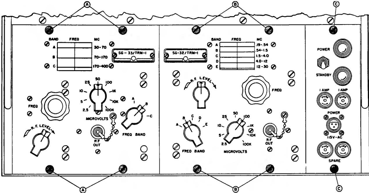
Figure 4-1. Front View for Removal of Signal Generators from the Equipment Case
