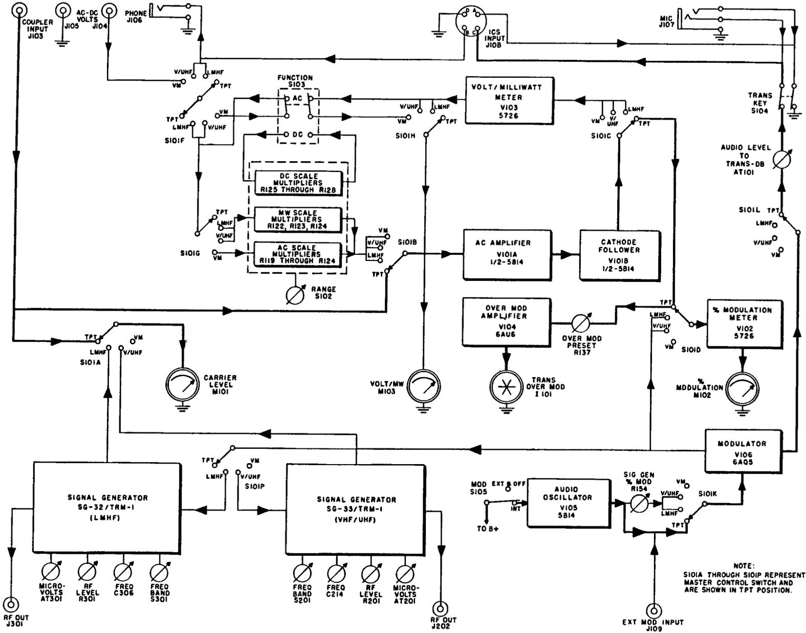
Figure 4-15. Master Block Diagram
