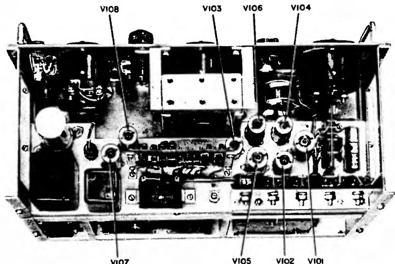
Figure 5-1. Test Set Subassembly TS-687/TRM-1, Tube Locations
