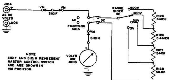
4-13. D-C Voltmeter, Simplified Schematic Diagram
