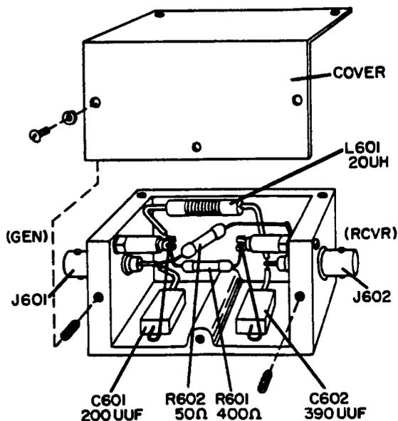
Figure 4-14. Adapter, Test MX-1652/TRM-1 (Antenna Simulator), Exploded View
