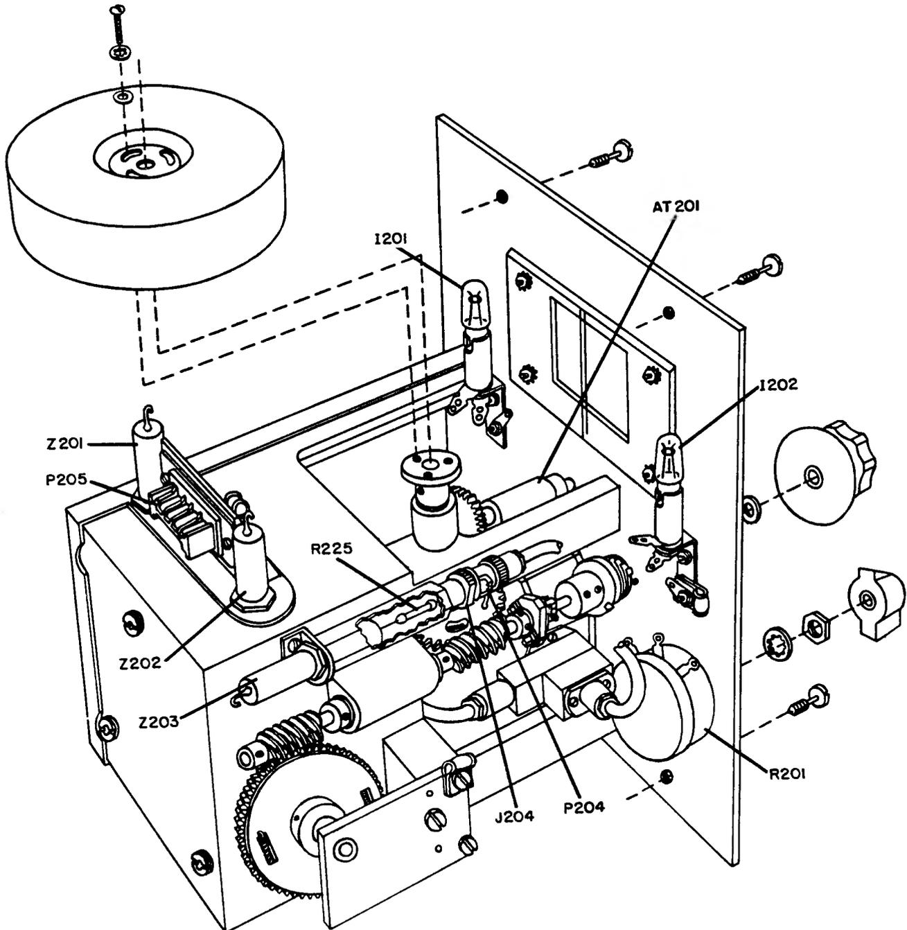
Figure 4-5. Signal Generator SG-33/TRM-1, Exploded View, Left Side
