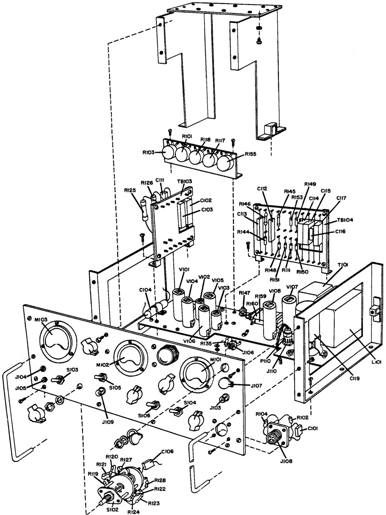
Figure 4-2. Test Set Subassembly TS-687/TRM-1, Exploded View
