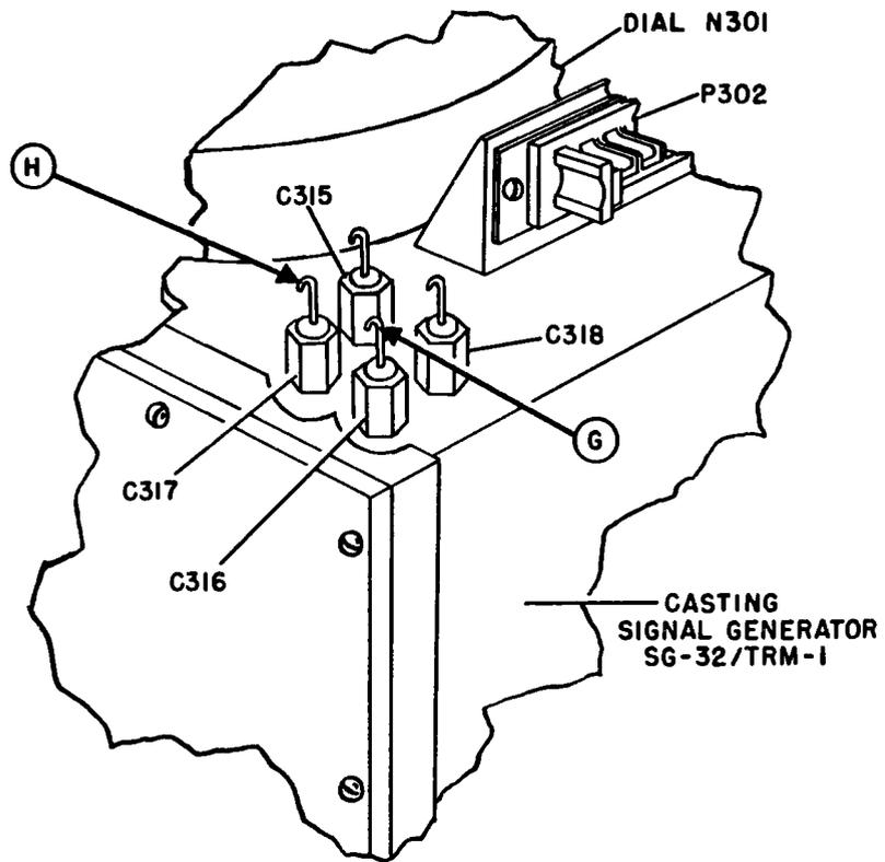
REAR OF CASTING SIGNAL GENERATOR SG-32/TRM-1
