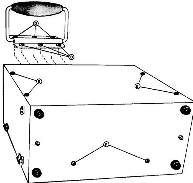
Figure 4-2. Rear-Bottom View for Removal of Test Set TS-687/TRM-1 from the Equipment Case
