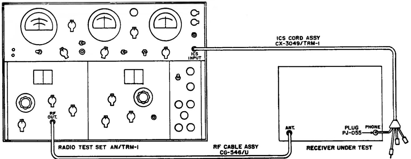
Figure 2-4. Typical Connections for Radio Receiver Performance Tests
