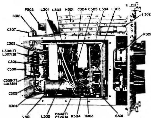
Figure 5-4A. Signal Generator SG-32/TRM-1, Location of Tubes and Component Parts
