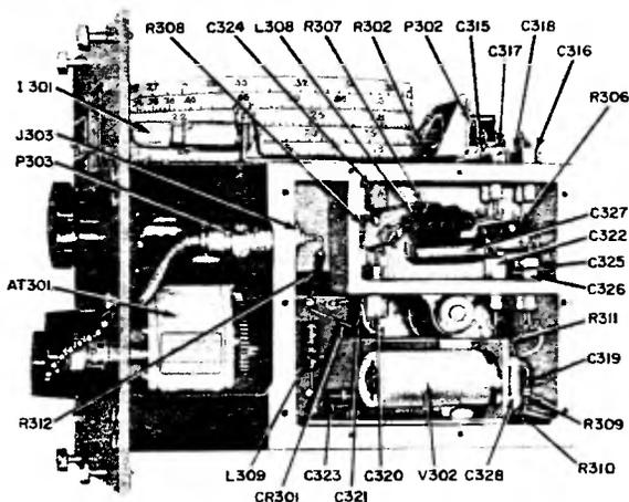
Figure 5-4B. Signal Generator SG-32/TRM-1, Location of Tubes and Component Parts
