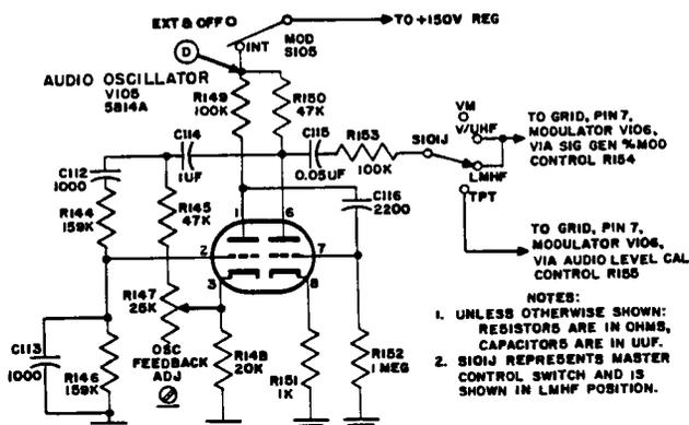
Figure 4-11. Audio Oscillator, Simplified Schematic Diagram
