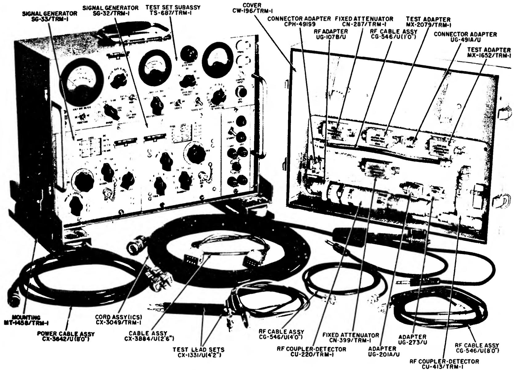
Figure 1-1. Radio Test Set AN/TRM-1
