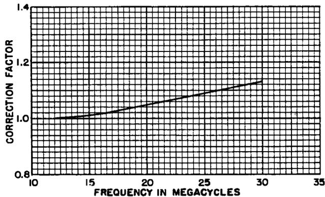
Figure 2-5. Correction Factor/Frequency Curve for Output Voltage on Band E of Signal Generator SG-32/TRM-1 (LMHF)
