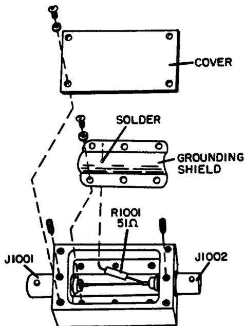
Figure 4-13. Adapter, Test MX-2079/TRM-1 (50 ohm Shunt), Exploded View
