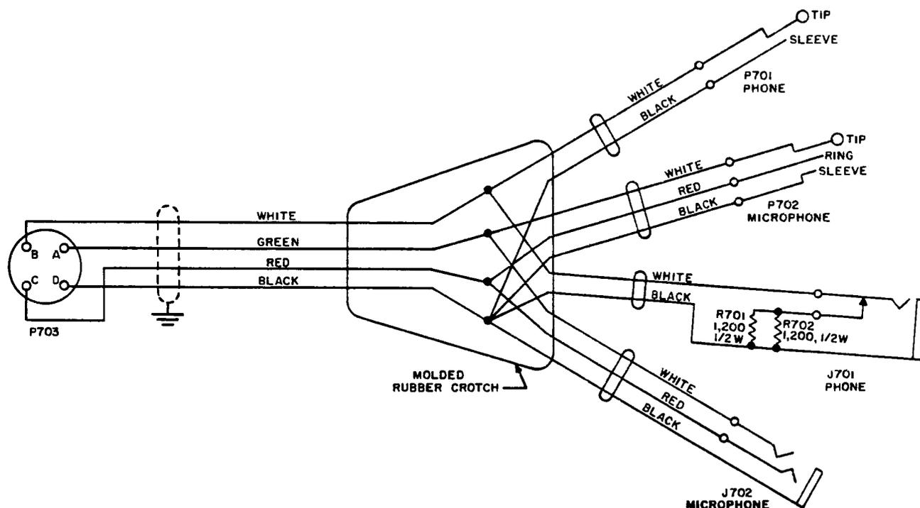
Figure 6-6. Electrical Cord Assembly CX-3049/TRM-1, Schematic Diagram
