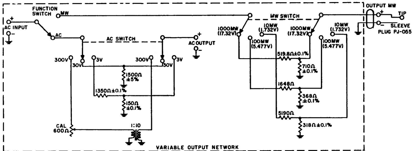
Figure 11-2. Set-up for Performance Test of AC Voltmeter and MW Meter
