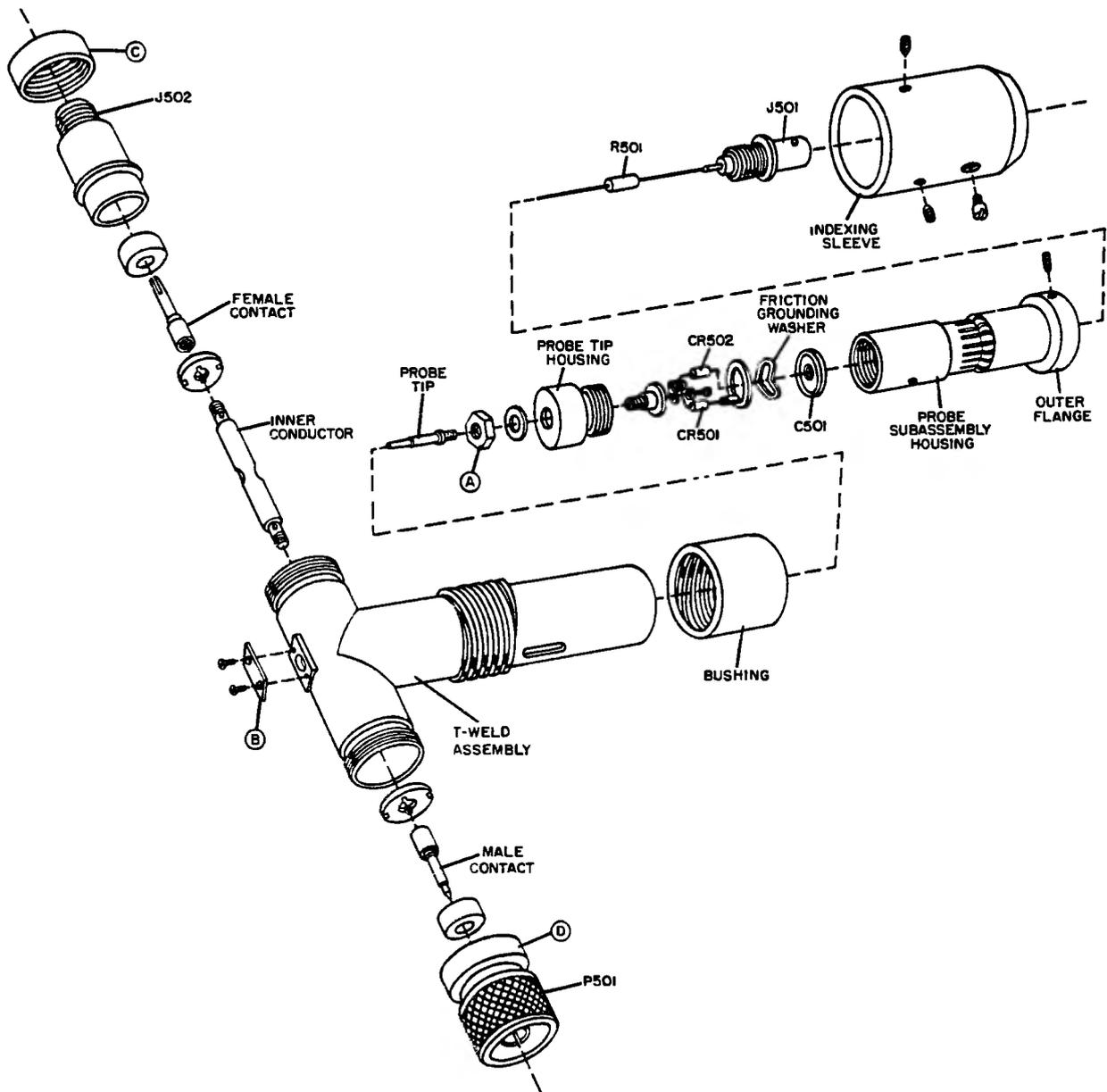
Figure 4-10. RF Coupler-Detector CU-413/TRM-1, Exploded View
