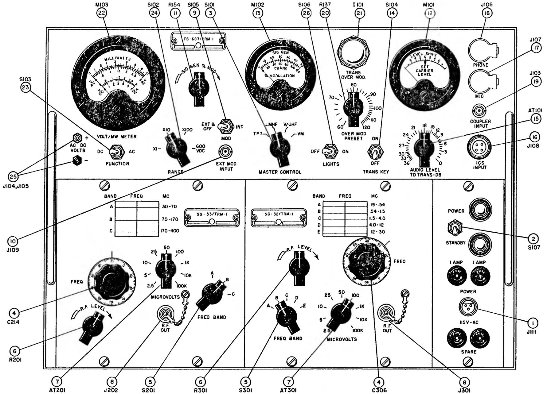
Figure 1-2. Operating Controls and Connectors, Radio Test Set AN/TRM-1
