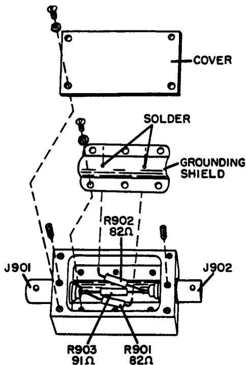
Figure 4-12. Attenuator, Fixed CN-287/TRM-1 (12 db), Exploded View
