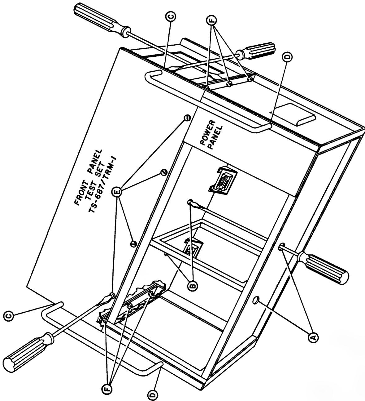
Figure 6-1. Disassembly for Test Set TS-687/TRM-1
