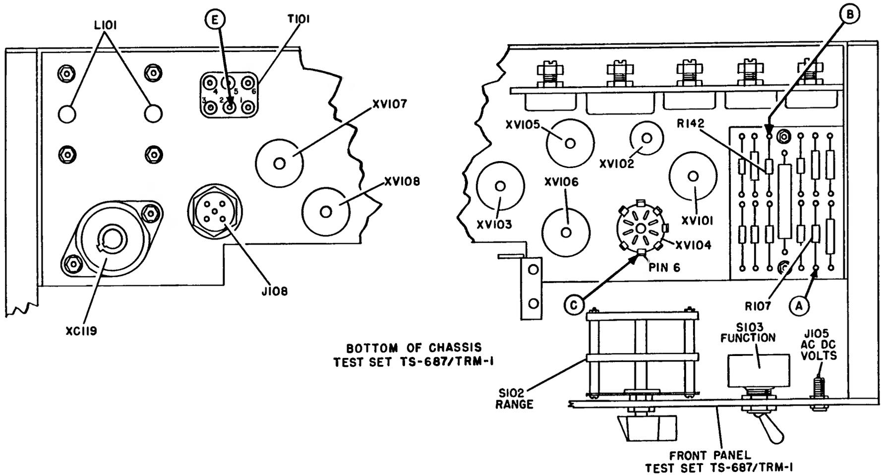
Figure 6-3. Location of Test Points, Bottom of Chassis, Test Set TS-687/TRM-1
