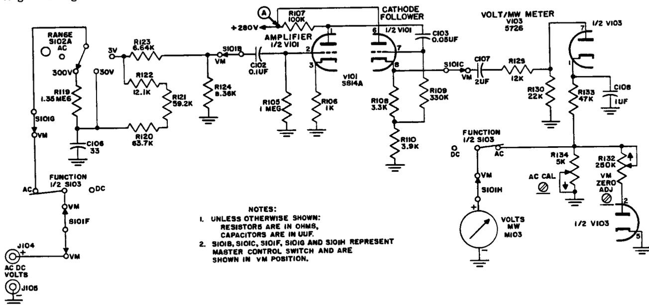
Figure 4-12. A-C Voltmeter, Simplified Schematic Diagram
