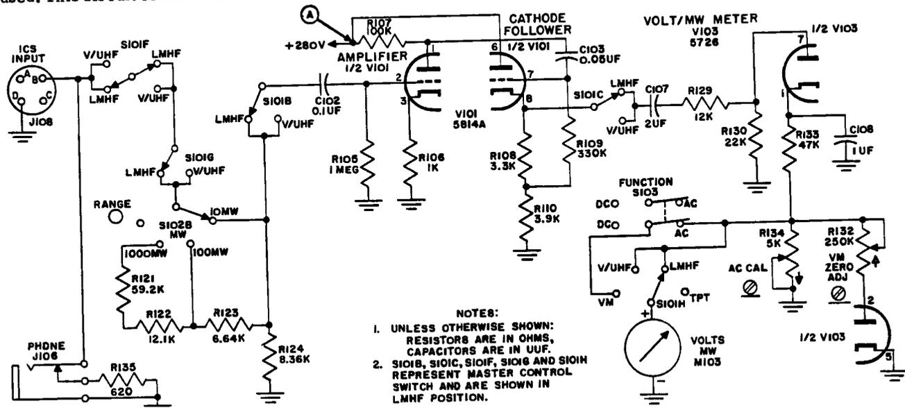
Figure 4-9. Milliwatt Meter, Simplified Schematic Diagram
