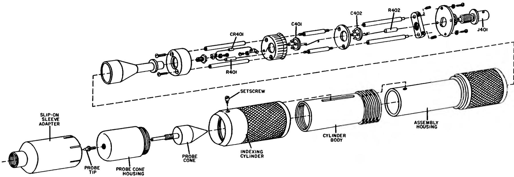
Figure 4-9. RF Coupler-Detector CU-220/TRM-1, Exploded View
