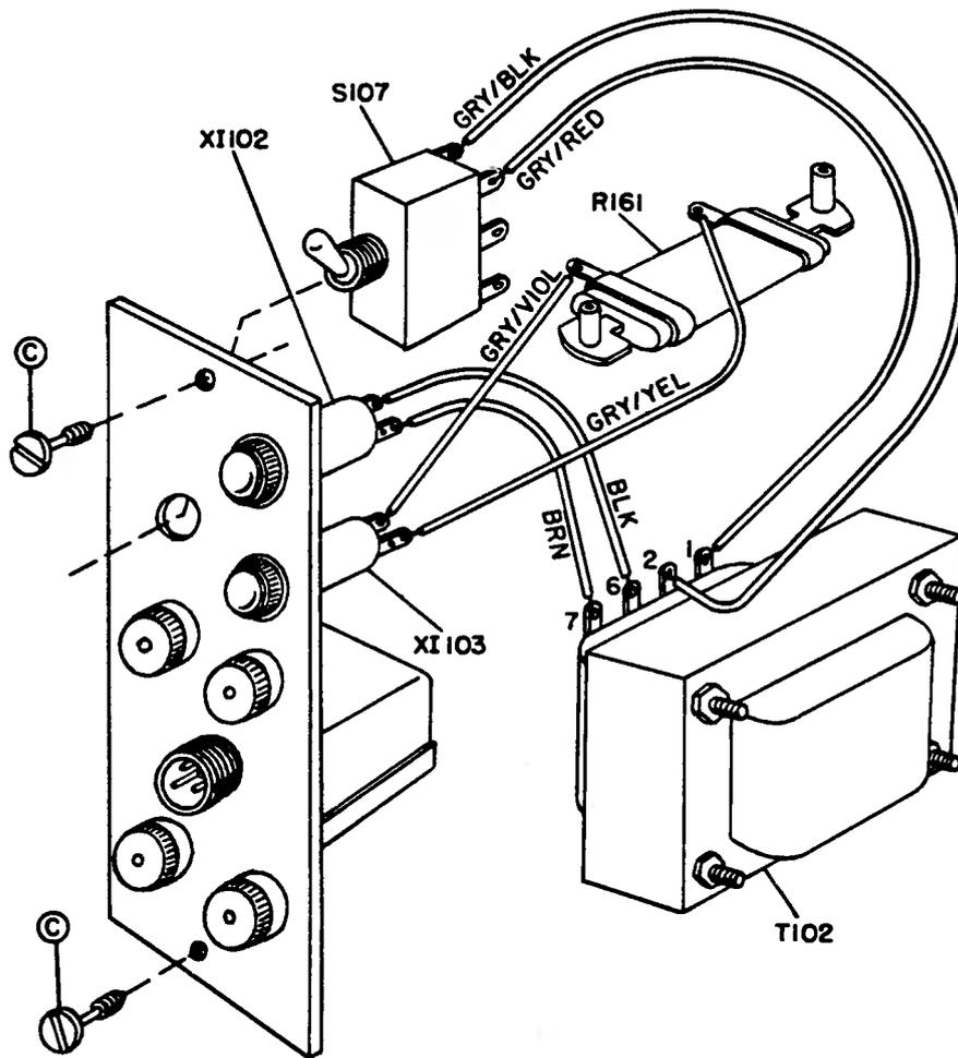
Figure 4-1. Connections from Power Panel to Chassis
