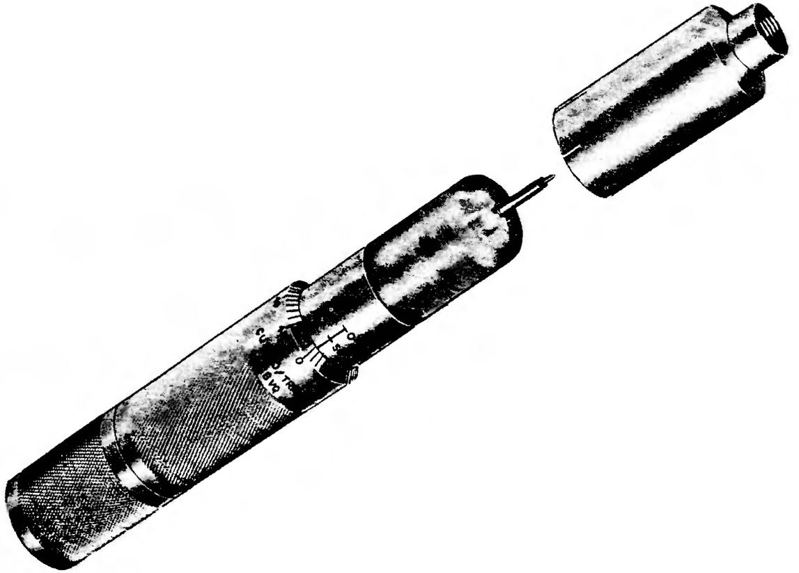
Figure 1-3. RF Coupler-Detector GU-220/TRM-1
