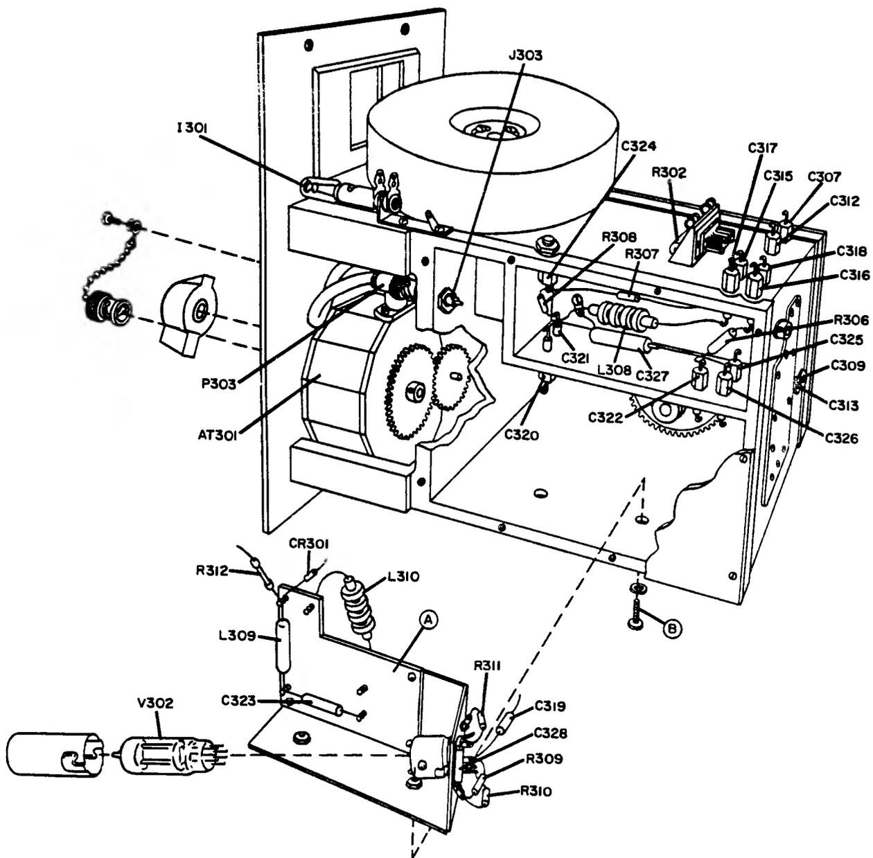
Figure 4-7. Signal Generator SG-32/TRM-1, Exploded View, Right Side
