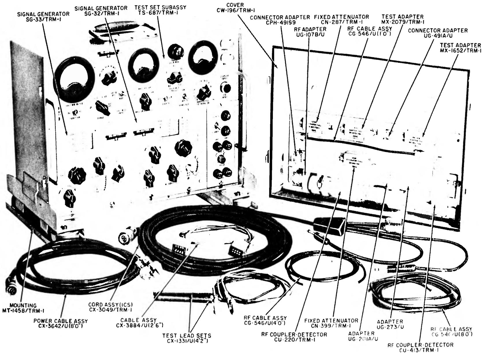
Figure 1-1. Radio Test Set AN/TRM-1, Equipment Supplied
