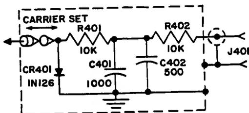
Figure 4-7. R.F. Coupler-Detector CU-220/TRM-1, Schematic Diagram
