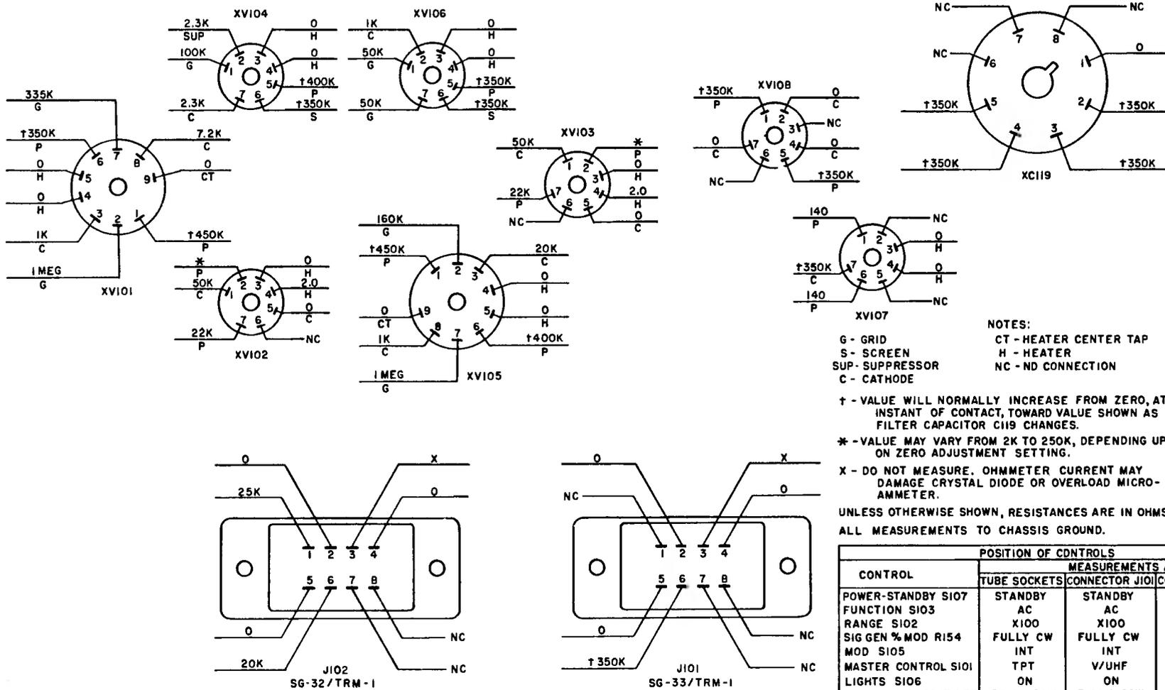
Figure 7-3. Radio Test Set AN/TRM-1, Resistance Chart
