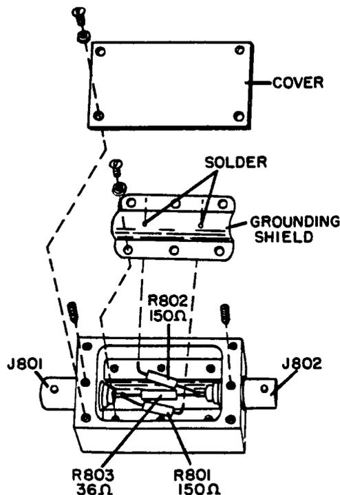
Figure 4-11. Attenuator, Fixed CN-399/TRM-1, (6 db), Exploded View
