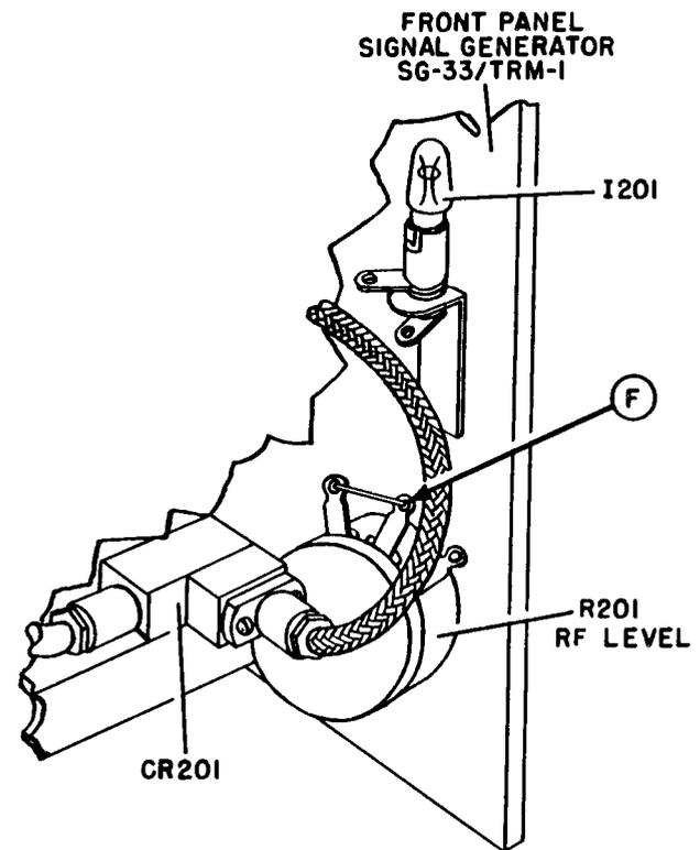
REAR OF FRONT PANEL SIGNAL GENERATOR SG-33/TRM-1
