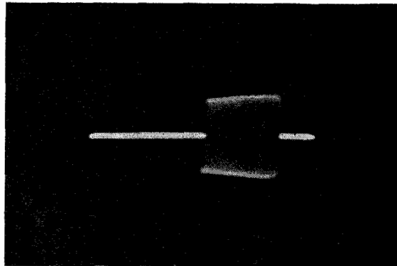
Fig. 28 Oscilloscope Pattern—CW Keying 100 W.P.M.
