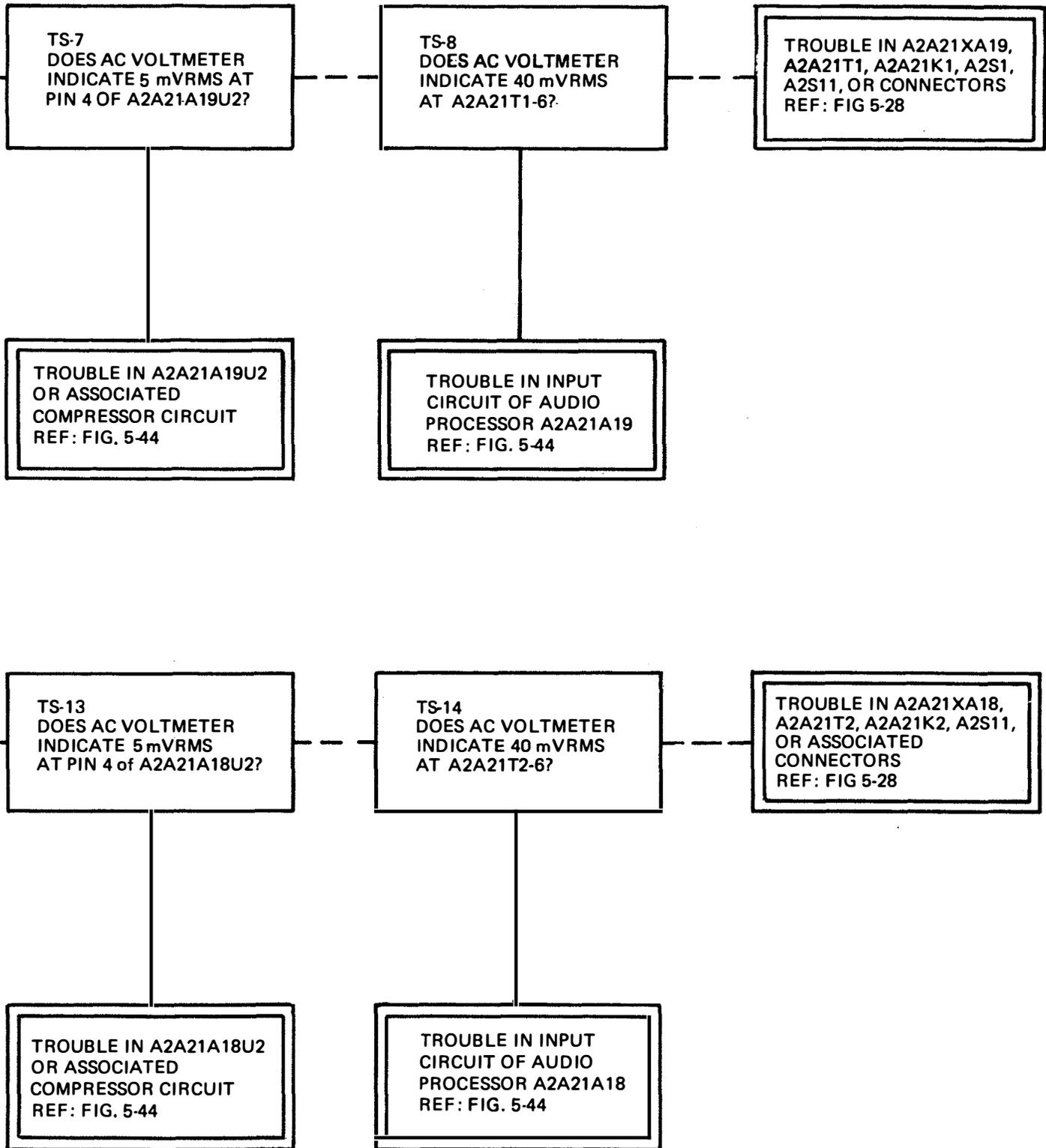
Figure 5-16. Normal Operation - Audio Amplification and Modulation, Voice Modes, Fault Logic Diagram, (Sheet 1 of 2)
