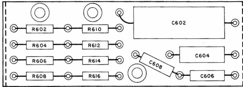
Figure 5-15. Channel B Network Assembly, Location of Rear Components
