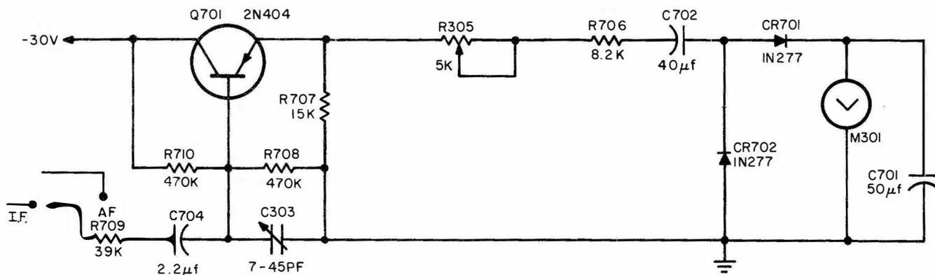
Figure 4-5. Meter Circuit, Simplified Schematic Diagram
