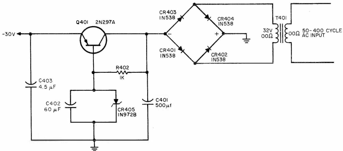
Figure 4-6. Power Supply, Simplified Schematic Diagram
