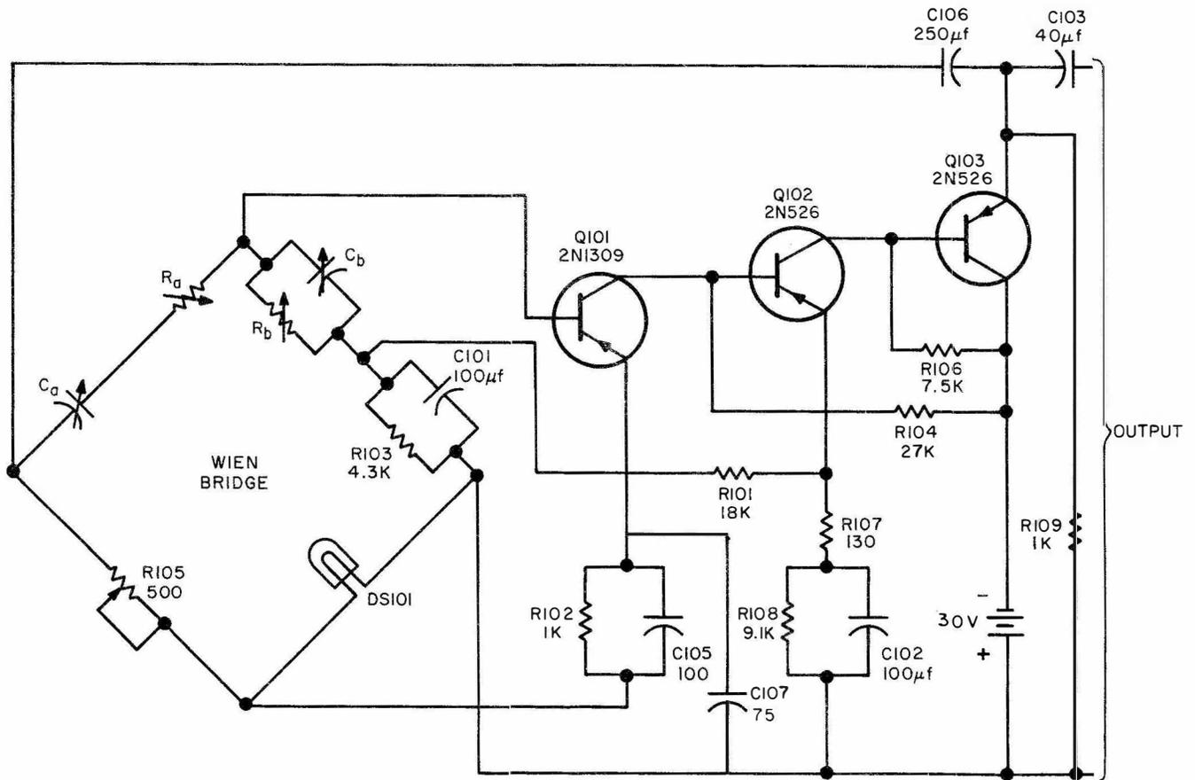
Figure 4-2. A.F. Oscillator, Simplified Schematic Diagram
