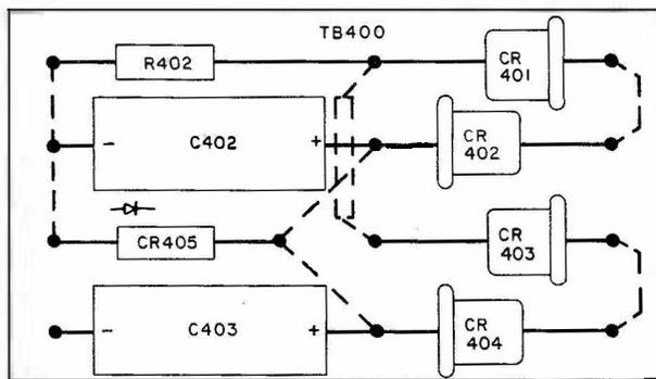
Figure 5-17. Power Supply Circuit Board Assembly, Location of Components
