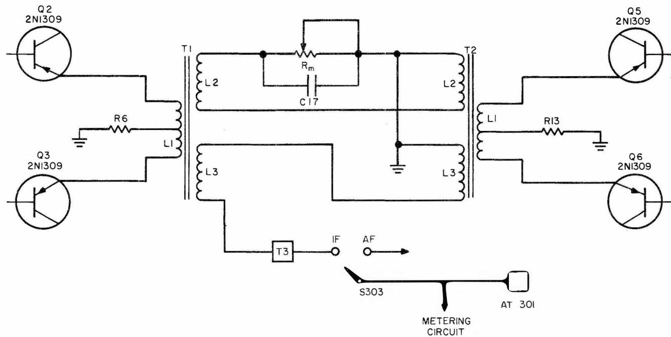
Figure 4-4. Hybrid Circuit, Simplified Schematic Diagram
