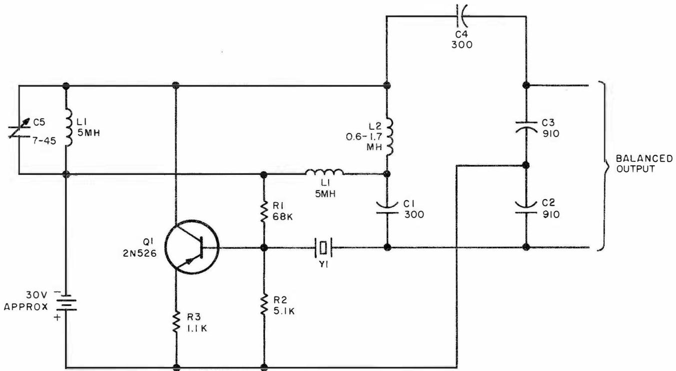
Figure 4-3. I.F. Oscillator, Simplified Schematic Diagram
