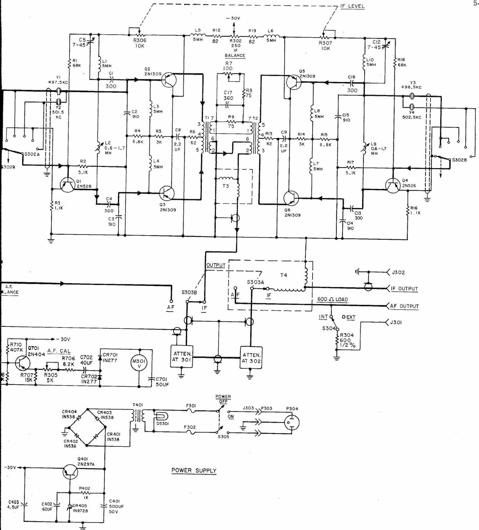
Figure 5-19. Signal Generator, SG-376A/U, Schematic Diagram
