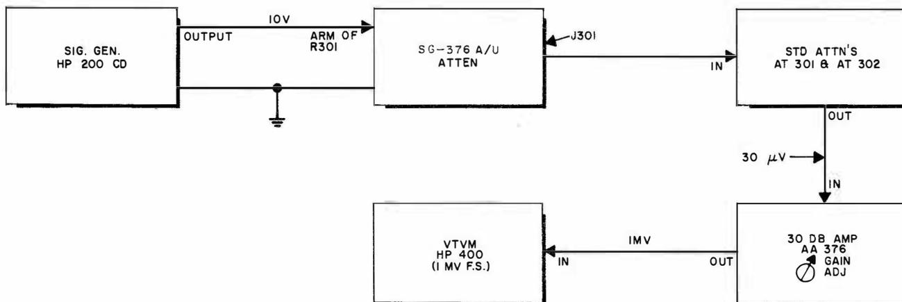
Figure 5-6. Set-up for Attenuator Test, Connection Diagram
