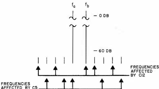
Figure 5-7. Effects of C5 and C12 Adjustment
