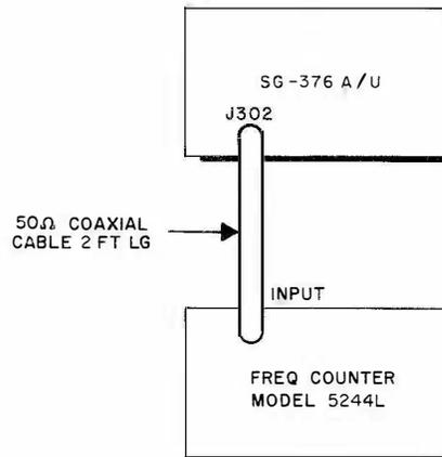
Figure 5-2. Set-up for I.F. Frequency Calibration Test, Connection Diagram
