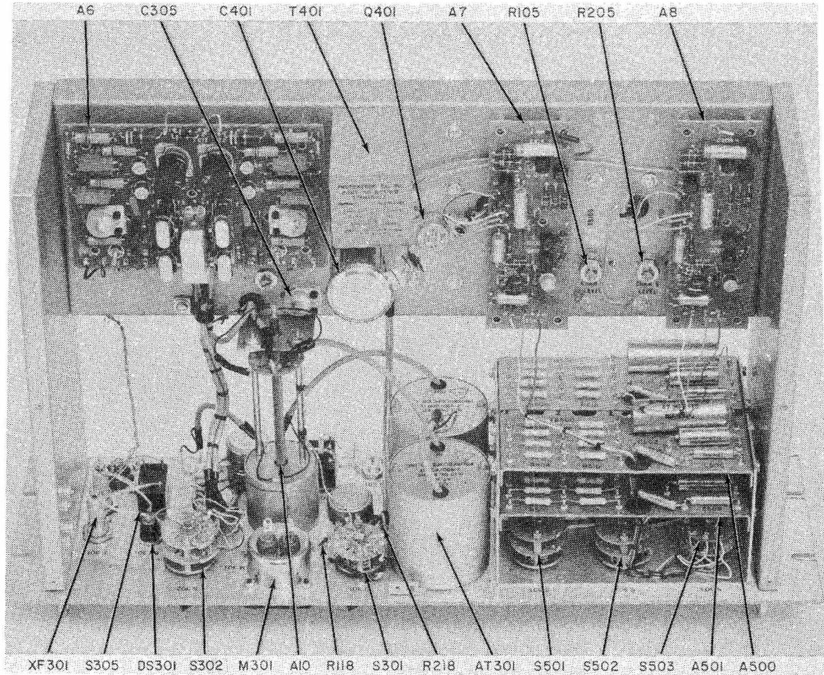
Figure 5-8. Signal Generator, SG-376A/U, Top of Chassis
