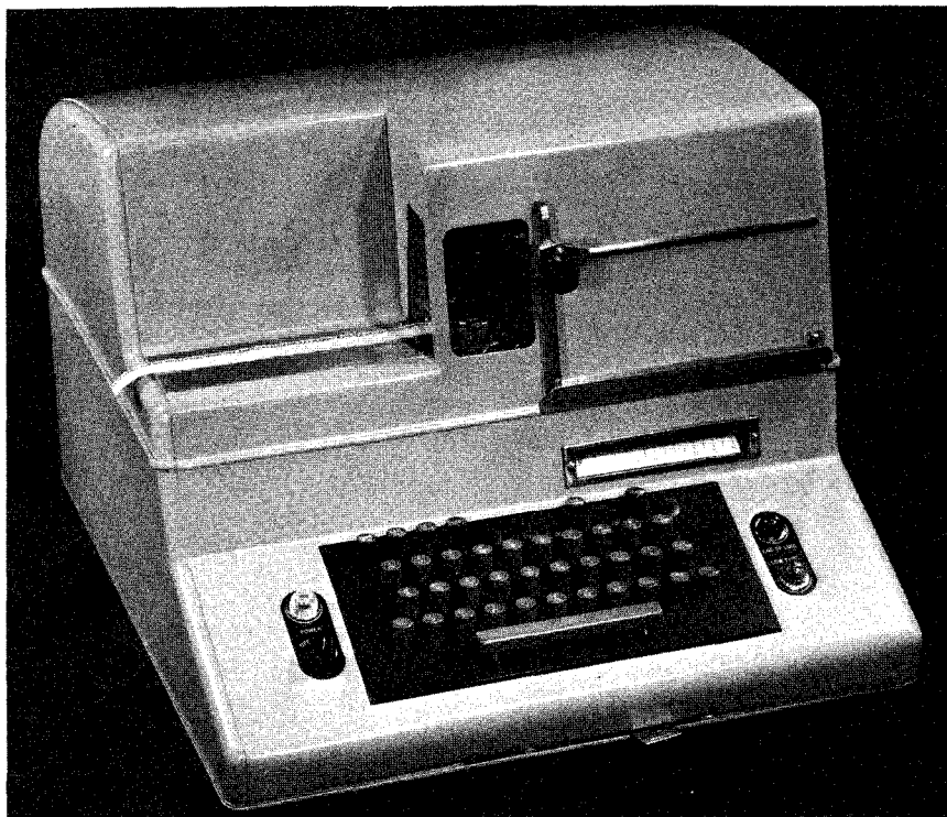
Figure 10-43. —Send/receive typing reperforator TT-253/UG.
