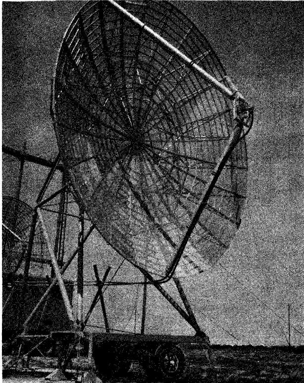
Figure 8-31. — Mobile tropospheric 30-foot scatter antenna.
