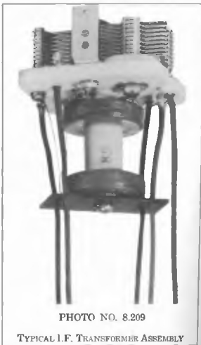
TYPICAL I.F. TRANSFORMER ASSEMBLY
