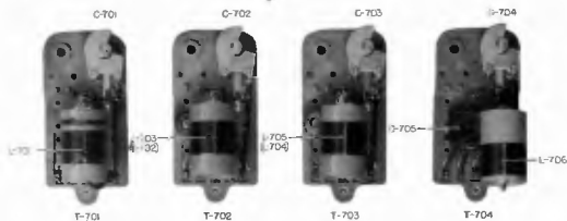
PHOTO NO. 17.14 R.F. TRANSFORMER SET No. 4
