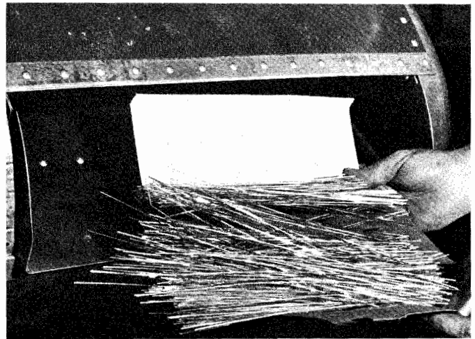
"WINDOW," USED TO CONFUSE ENEMY RADARS DURING BOMBING RAIDS OVER GERMANY
