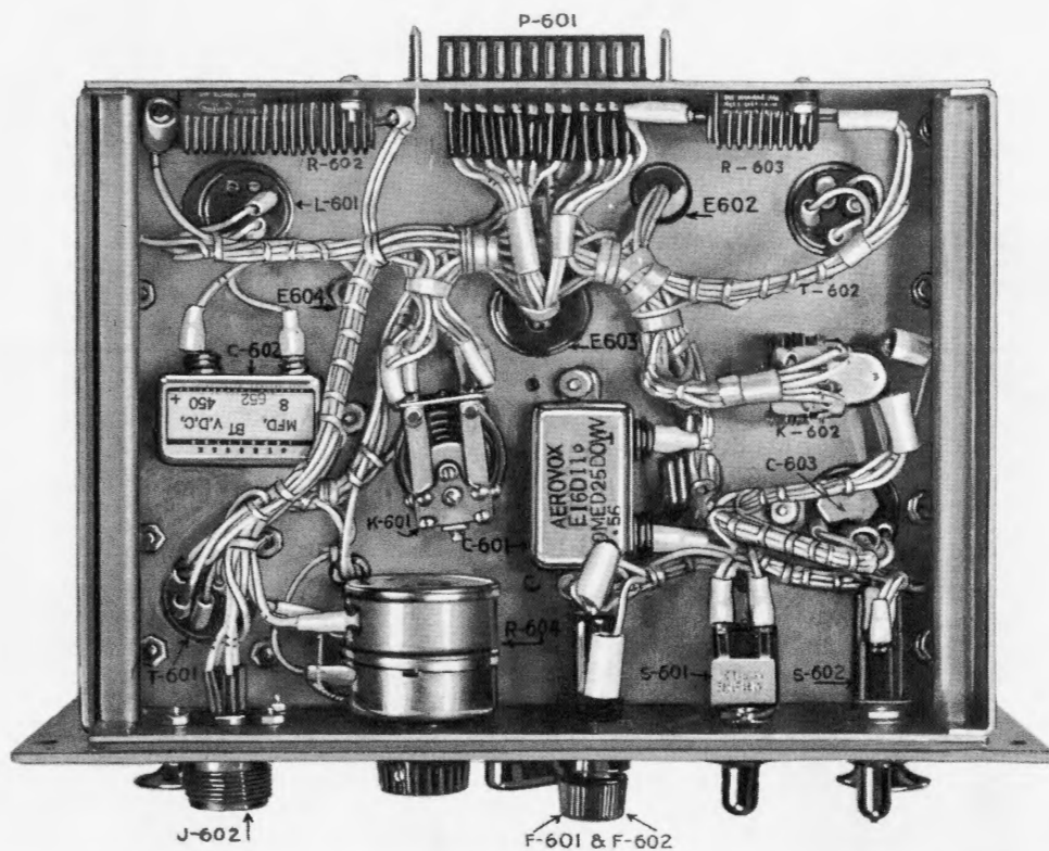
Figure 5-2. Adapter, Control, Location of Test Points, Bottom of Chassis
