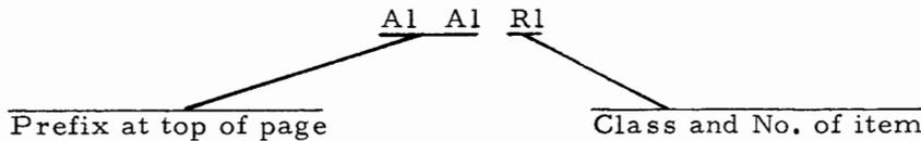
Read as: First (1) resistor (R) of first (1) subassembly (A) of first (1) assembly (A). Top of page prefix A1A1 added to class and number of Item R1.
