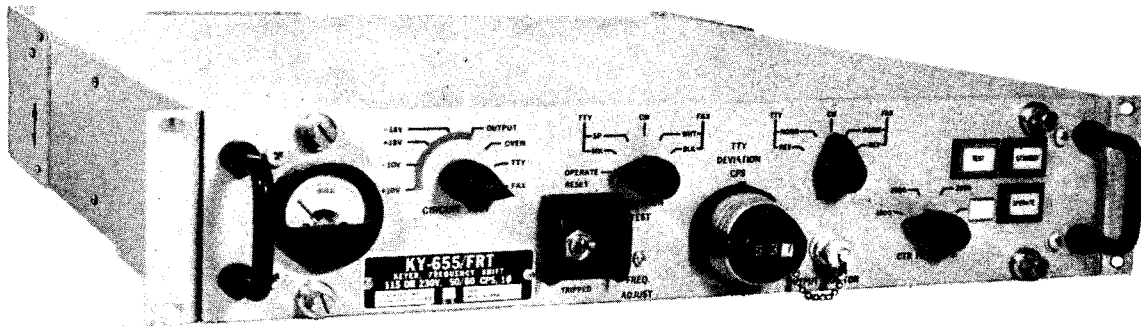
Figure 1-1. Keyer, Frequency Shift KY-655/FRT
