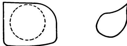
Figure 7-3. Oscillograms — RF Oscillator O-91A/FRT-5, 100-Kc Phase Splitter Circuit Phase Relations
