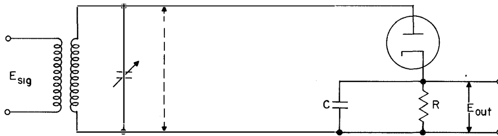
(a) Circuit of Simple Diode Detector
