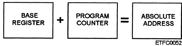
Figure 5-8.—Block diagram of an operation to determine an absolute address.
