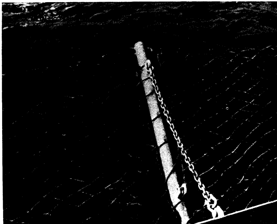
b. Metallic Safety Nets, Chain and Cable Figure 8-13. Typical Intermodulation Product Sources
