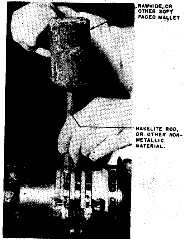
FIGURE 2.—Method of improving the concentricity of the slip rings.
