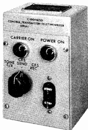
Figure 1-1 Transmitter Teletypewriter Control C-1004B/SG, Identification of Front Panel Controls
