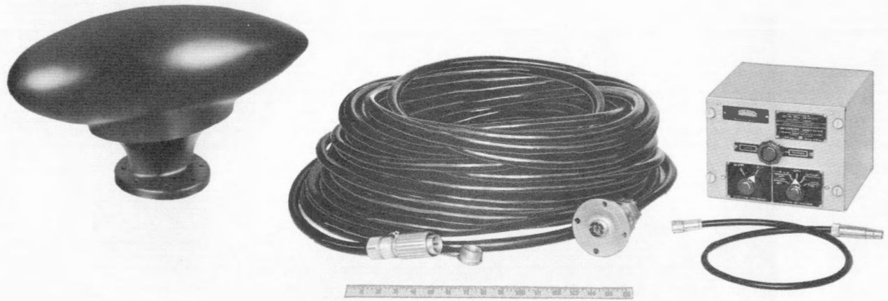
Figure 1-1B. Navy Model AT-317C/BRR VLF Loop Antenna System Relationship of Units.
