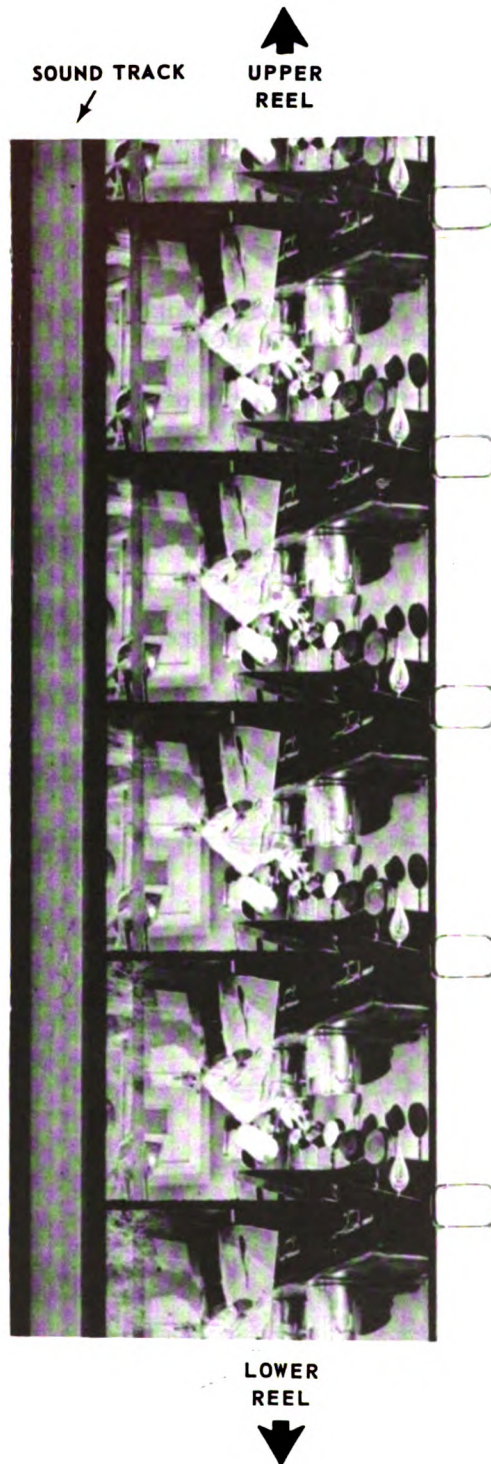
Figure 11-6.—Section of 16-mm sound motion picture film.
