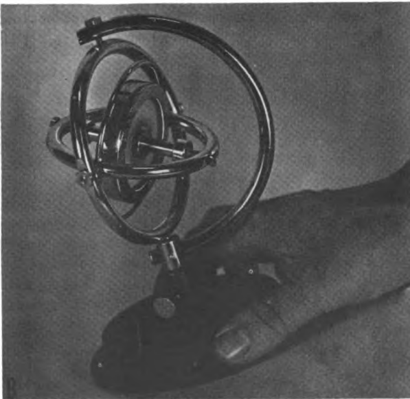
Figure 10-3.—Rigidity of plane of spinning gyroscope.
