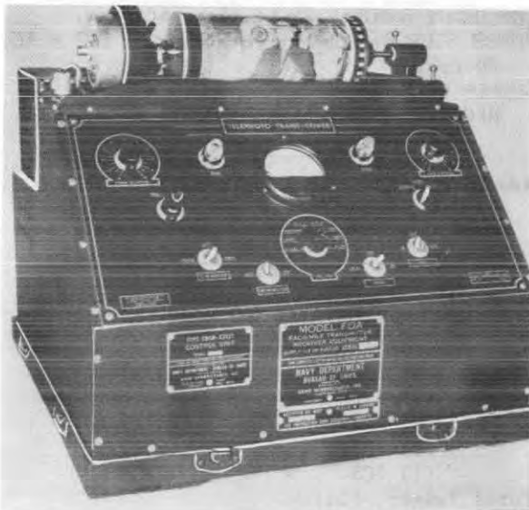
Transmitter-Receiver Equip FOA,FOC
