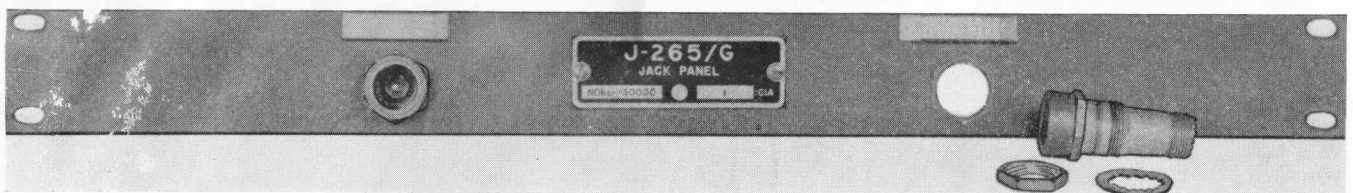
Figure 1-25. Jack Panel AN Type J-265/G, Front View With One Adapter AN Type UG-294/U Removed
