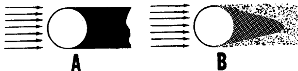
Figure 6-3. --Bending effect caused by diffraction.
