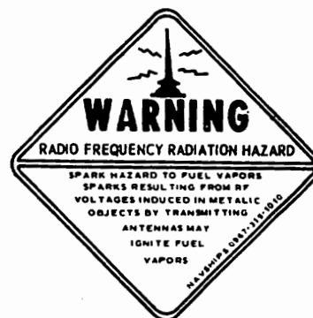
LOCATION: AT FUEL HANDLING AREAS WHICH ARE SUBJECTED TO RF RADIATION.
