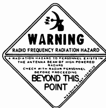
LOCATION: AT EYE LEVEL AT THE FOOT OF ALL LADDERS OR OTHER ACCESSSES TO ALL TOWERS, MASTS AND SUPER-STRUCTURES WHICH ARE SUBJECTED TO HAZARDOUS LEVELS OF RADIATION.
