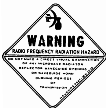
LOCATION: ON RADAR ANTENNA PEDESTALS.
