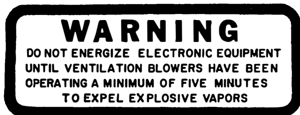
Figure 2-12.—Warning plate for electronic equipment installed in small craft.
