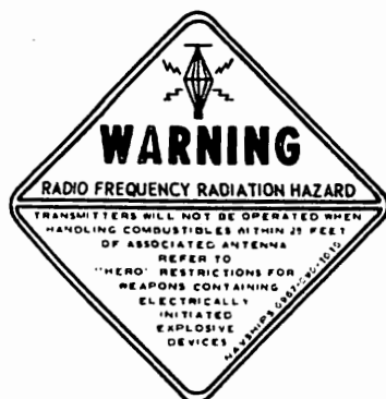
LOCATION: IN RADIO TRANSMITTER ROOMS IN SUITABLE LOCATION FOR FULL VIEW BY OPERATION PERSONNEL.
