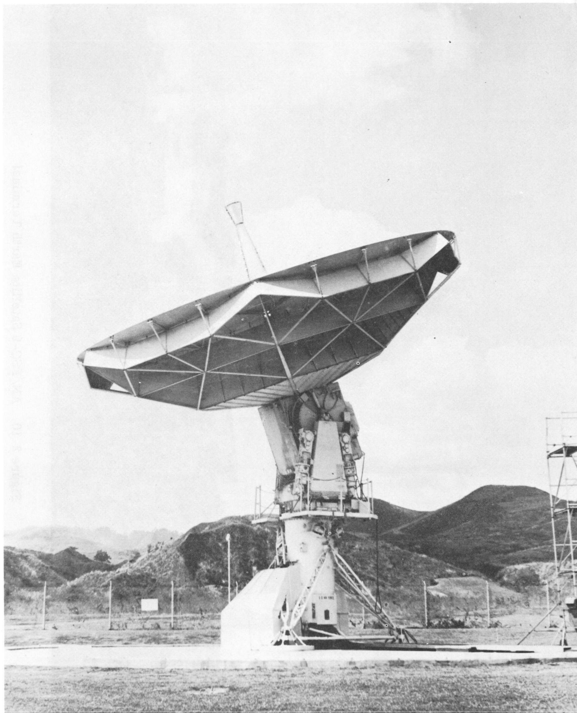
Figure 2-11. AN/MSC-46 Antenna and Pedestal
