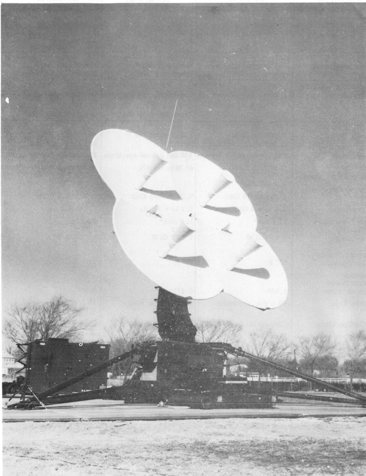
Figure 2-12. AN/TSC-54 Satellite Communication Terminal
