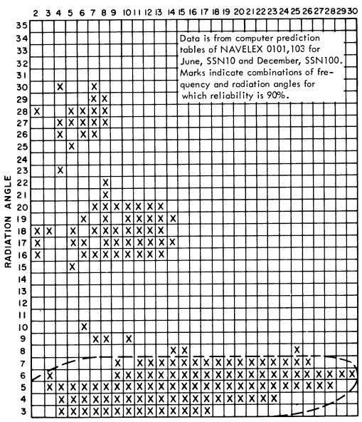
Figure 5-1. Radiation Angle/Frequency Matrix
