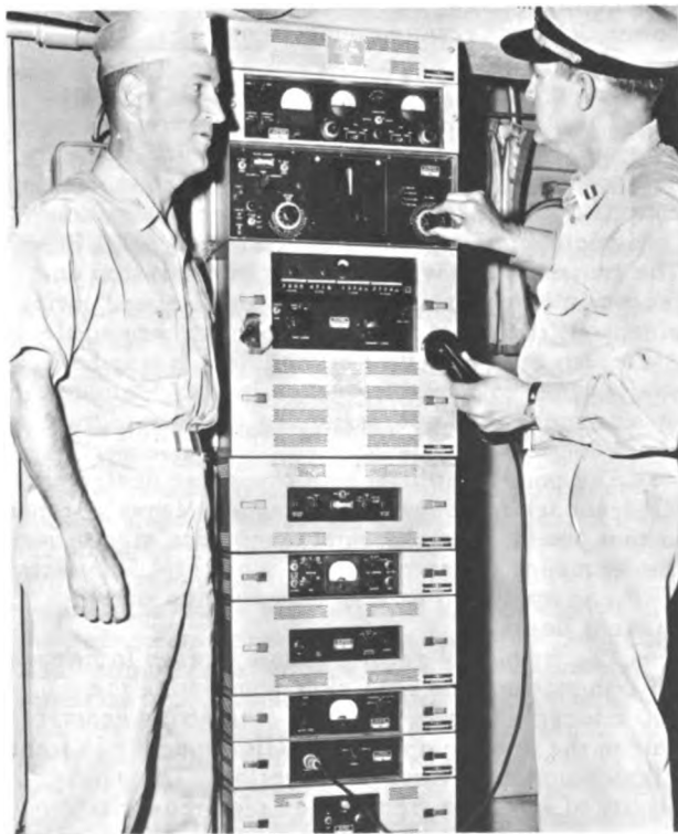
AN/URC-32 HF SSB transceiver is demonstrated to Capt. Harold G. Bowen, Jr. (left), Commander of the USS Northampton, by the ship's Electronics Material Officer, Lt. H. Criner.
